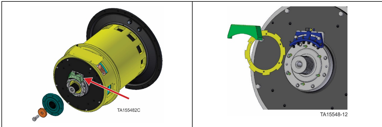
Figure 13. Motor RPT assembly (typical)
